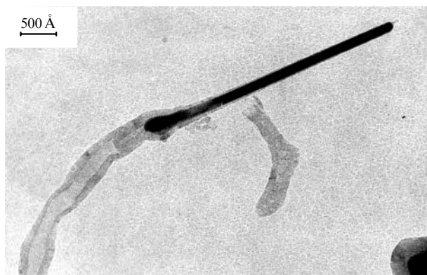
Figure 11. A micrograph of the filamentous carbon formed from methane on the Ni–Cu/MgO catalyst at 973 K.
