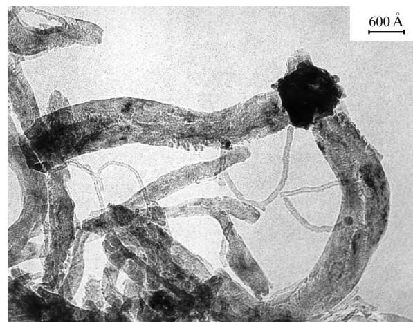
Figure 7. Morphology of the carbon formed from methane on the block particle of Ni–Cu alloy after a 5-min relaxation at 873 K.
